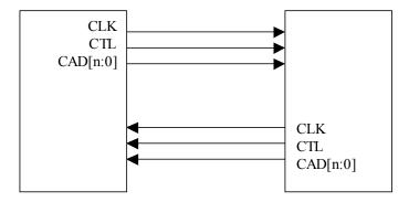
Figure 1. HyperTransport<sup>TM</sup> I/O Link
