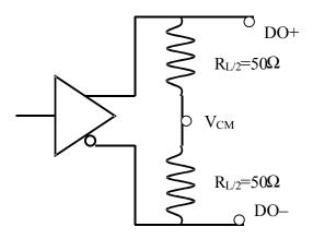
Figure 13. DC Output Reference System Load
