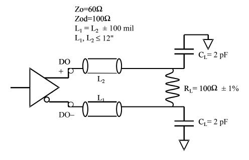
Figure 19. AC Reference System Load for Links Above 800 MT/s
