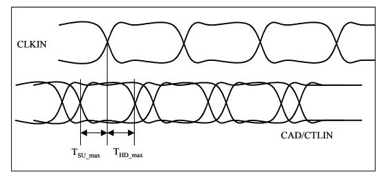
Figure 27.  $T_{SU}$  and  $T_{HD}$
