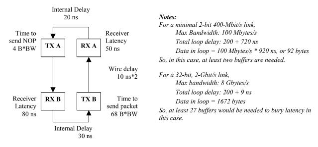
Figure 4. Example Data Buffer Sizing Calculation
