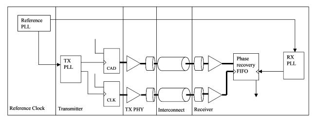
Figure 30. Representative Transmitter and Receiver
