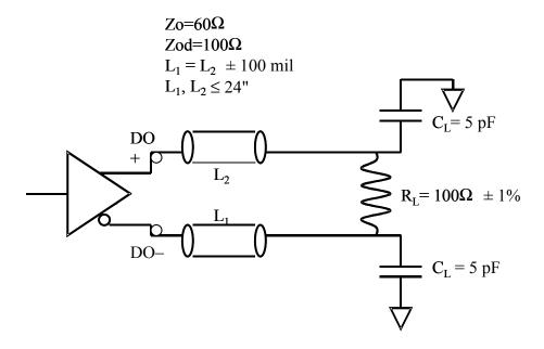
Figure 18. AC Reference System Load for Links up to 800 MT/s
